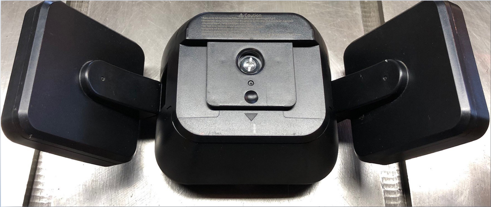
Back of motion-sensitive lamp, showing plastic bracket
