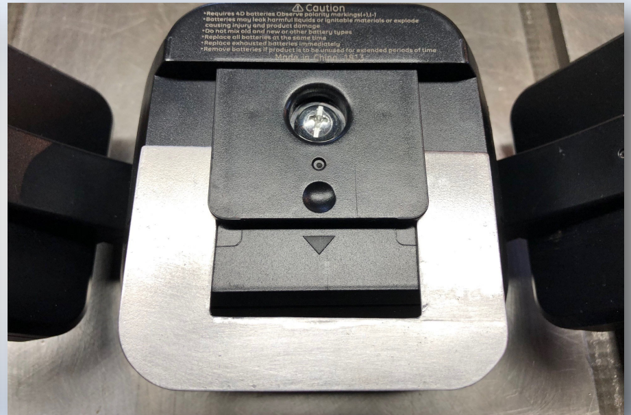
Test-fitting the bracket (mated about half-way).
