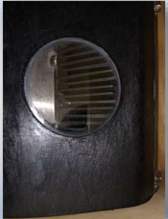
Looking into right window with capacitor fins fully meshed.
