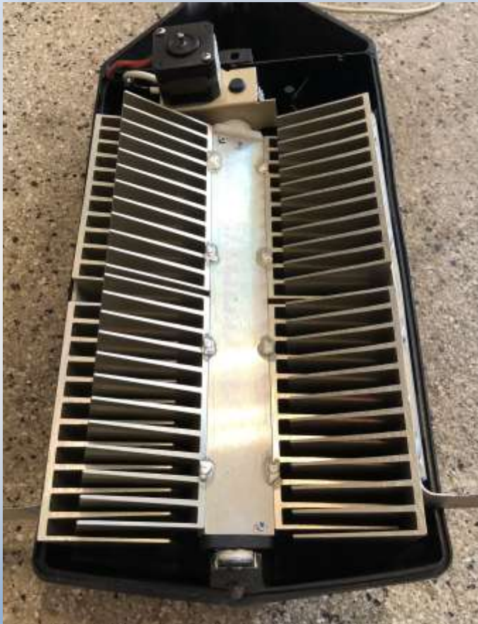
Butterfly capacitor, made from welded heat-sink material.
