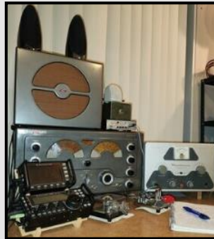
W0VLZ's National NC183 with a Heathkit DX40, a 1950s novice station, and an Elecraft KX3 with PX3 panadapter, a current SDR station.
