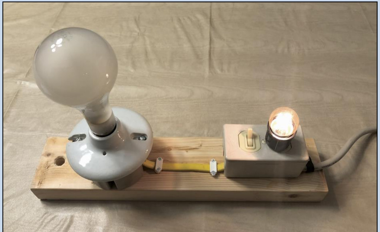
The DUT is the small bulb on the right. (In this case, there is not even enough current to "light" the limiter-bulb, which is the 300W incandescent on the left.)
